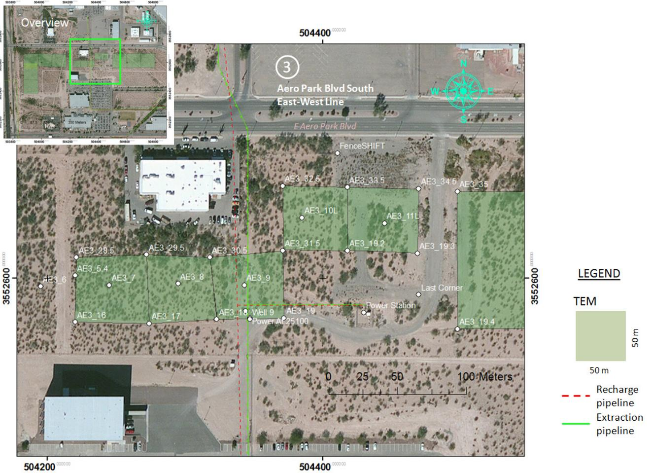
Fig 2.6 Five 50 m x 50 m TEM loops at approximately the center of the Aero Park Blvd east-west line.
