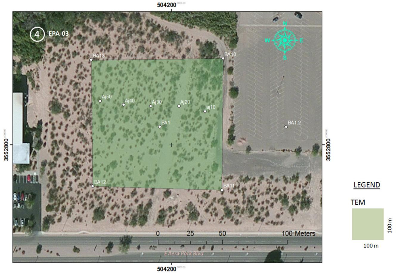
Figure 2.9 100 m x 100 m TEM loop at the EPA-03.
