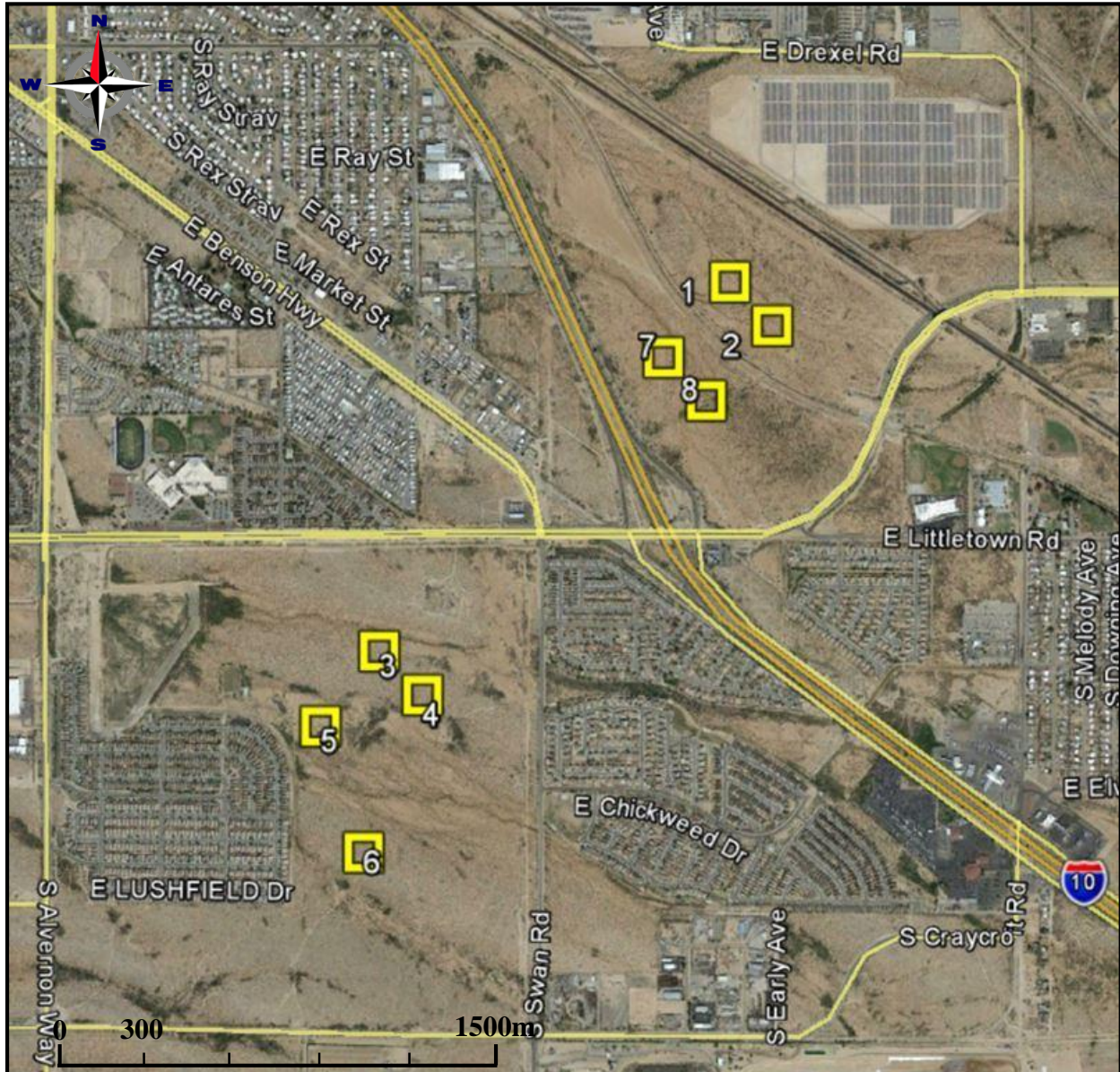
Figure 6.1 TEM survey stations. The loop size for TEM survey is 200m × 200m. There are 8 loops in the survey area.
