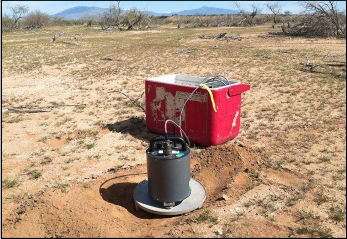
Figure 5.2 Seismometer in the field taking measurements. The battery is housed in the cooler.
