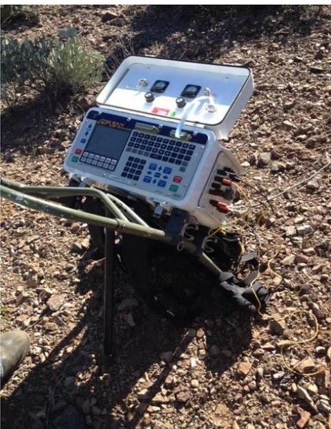
Figure 3.1. Zonge GDP-3224 multi-function receiver attached to the TEM/3 receiving antenna (not shown).
