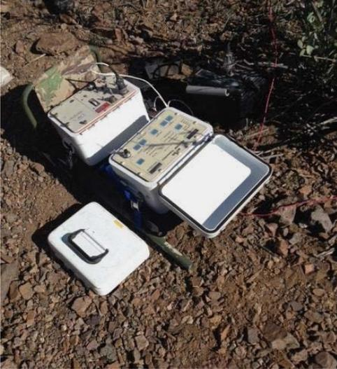
Figure 3.2. Zonge XMT-32 transmitter controller and NT-20 NanoTEM transmitter attached to copper loops (red wires).
