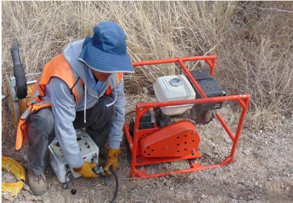
Figure 3.1. 3kW ZMG-9A gas powered generator.
