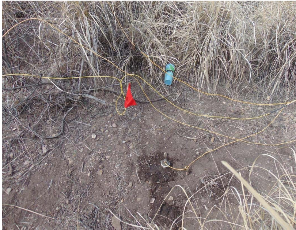
Figure 3.5. Porous pot receiver electrode.
