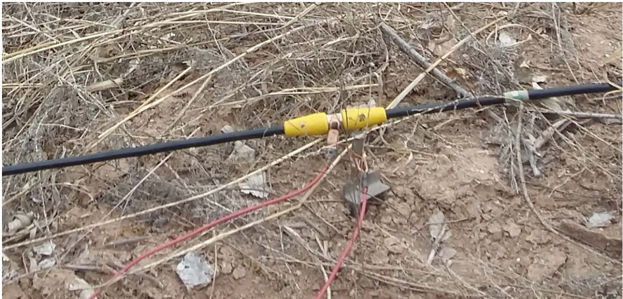
Figure 4.1a. Transmitter/receiver cables had takeouts every 6 meters. These takeouts were connected to electrodes with the copper clips, also shown in this photo. These arrays were used to collect all of the information for the Schlumberger and alternative Wenner arrays.
