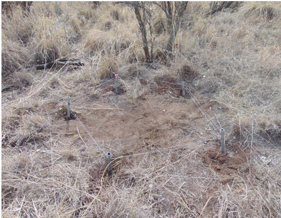
Figure 3.6. Pentagon of metal stakes used as a transmitting electrode.
