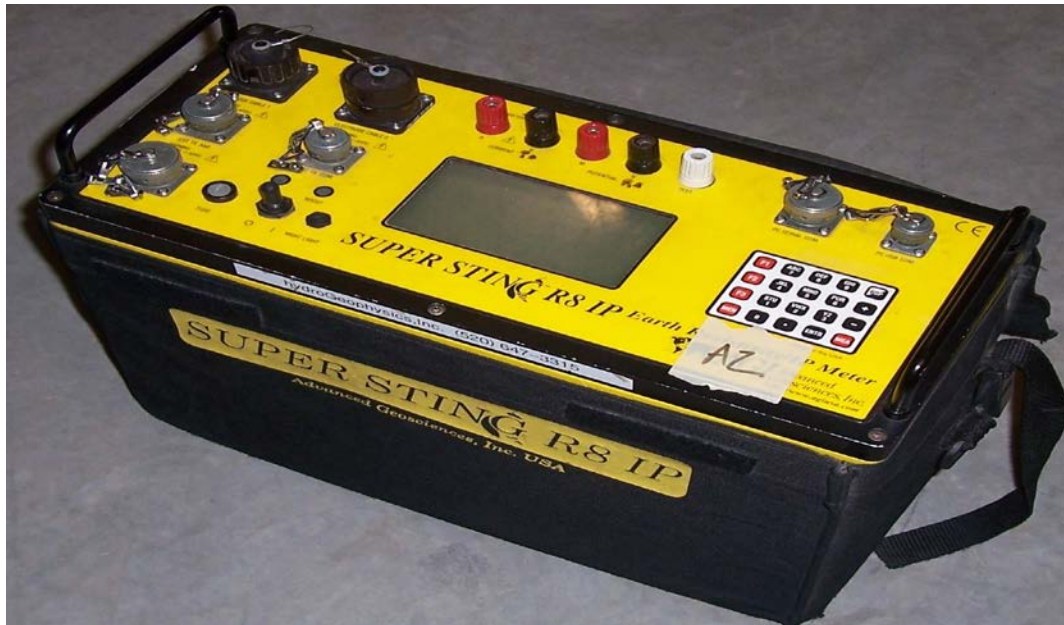
Figure 4.1b. SuperSting control unit. Using a pre-created command file, this unit controls which electrodes are being used as transmitters and which are being used as receivers. This console also collects and stores all of the data collected in each line. This console is battery powered, and for this project standard car batteries were used. (Source: hgiworld.com)
